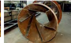
Feed trunnion liner
