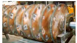
Clinker breaker discs
