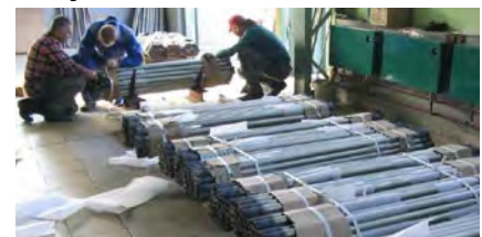
Wearfaced Boiler Tubes
