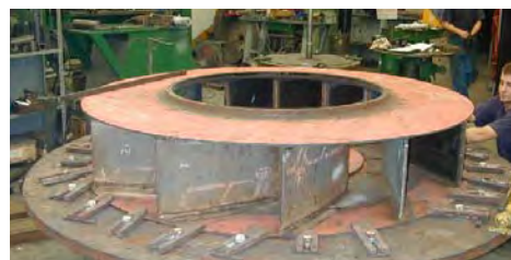
Fan built with Wear Resistant CDP
