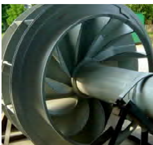
Wear Resistant Fan built with CDP
